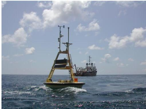
*Texas Automated Buoy System buoy for oil spill response (Credit: TAMU GERG)*
